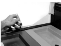
Figure 31: Lubricating The Main Frame
