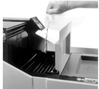
Figure 19: Loading Fixer Solution (Note the protective baffle by using the fixer evaporator cover between solution trays when pouring fixer. Use the same procedure with the cover for developer when pouring the developer).
