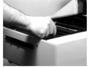
Figure 30: Pulling Out Drain Plug
