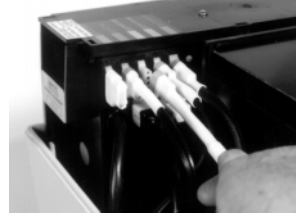
Figure 12: Connecting cable to light blue receptacle marked SOL.
