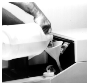
Figure 18: Filling Replenisher Tanks
